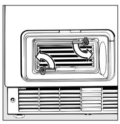
■ Turn both levers on the heat exchanger so that they are vertical
